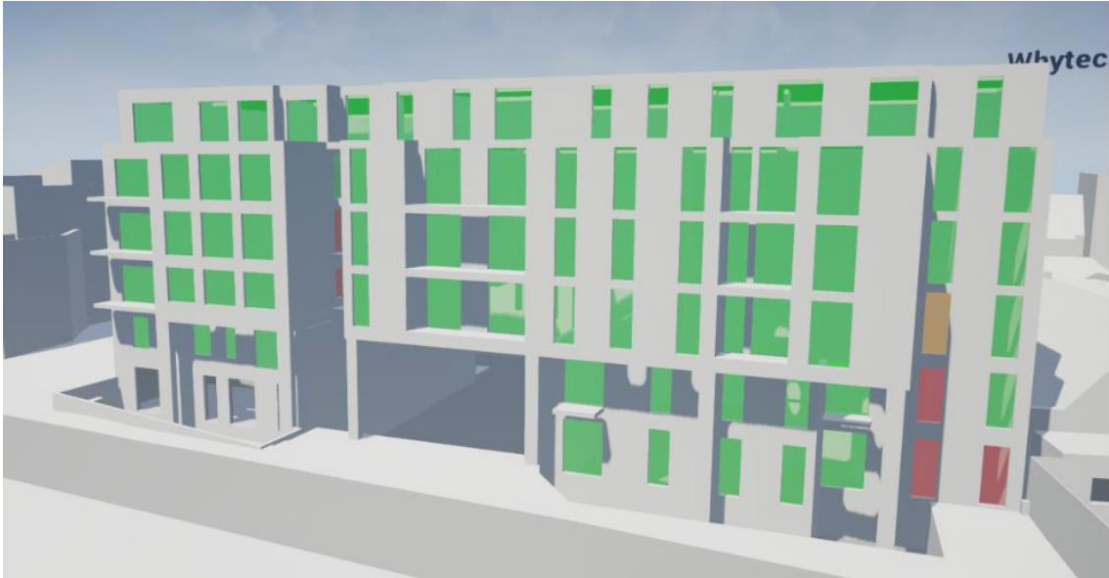
Figure 31 – Colour coded model showing retained VSC values once impacts of balconies/overhangs is removed. Green windows are those with retained values over 18% VSC.
